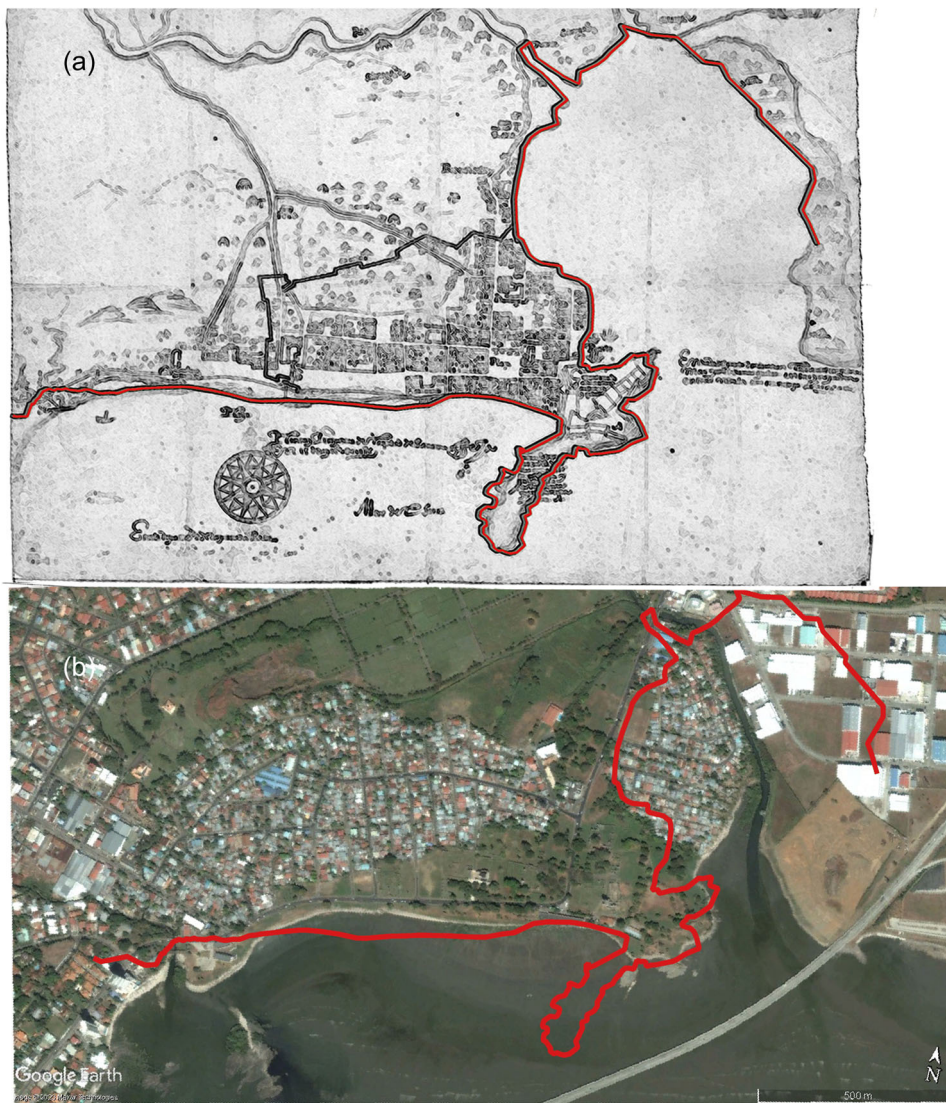
FIGURE 8 Evidence of erosion along the coastline includes the disappearance of the peninsula that Antonelli drew in 1586 (a), and whose remains were visible underwater in the aerial photo from 2004 (b). Covering these remains, the mangrove regrew after 2006. The irregular form of the historical map (a) is a consequence of the rectification process to adapt the image to reality.
